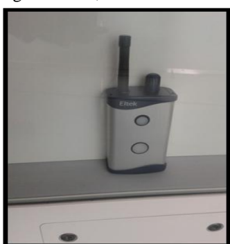
Image 4: This kind of hand-held light meter can be used in the galleries Source: www.spri.cam.ac.uk
